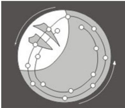
Ball mill rotary speed is normal
